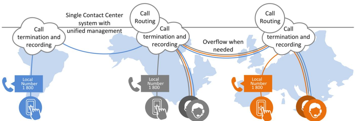
Figure 4: Global contact center operation using a single cloud contact center vendor with multi-tenants and multi-clouds
