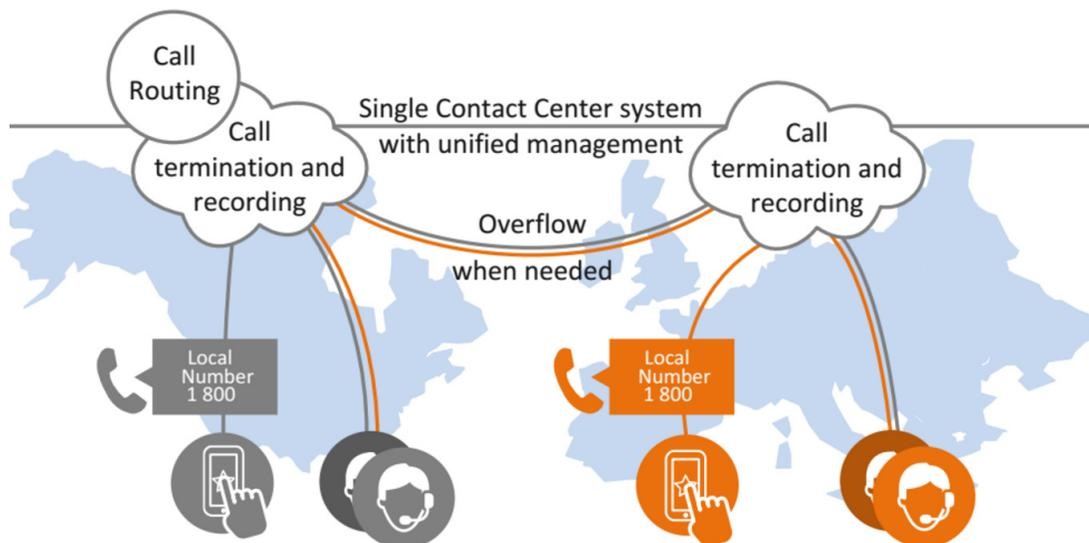
Figure 3: Global contact center operation using a single cloud contact center vendor with Edge Device functionality
